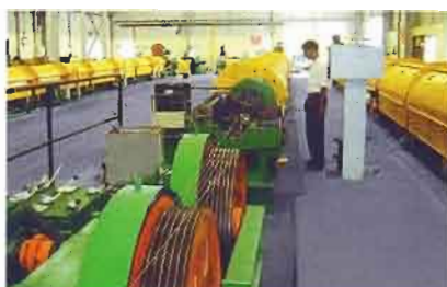
View of the Wire Spooling & Long Stranding Machines (18 Bobbin, 25 Bobbin & 3 no. 36 Bobbin)
